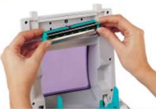
▼ Tool-less printhead replacement
